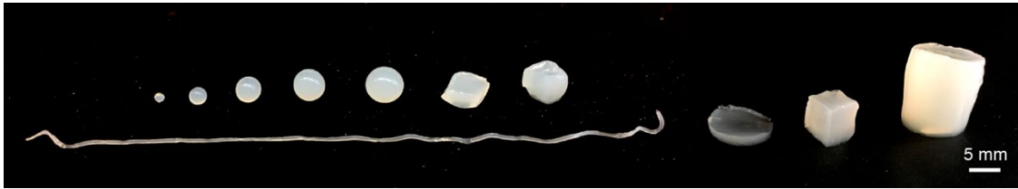
Figure 52 | Alginates in various geometries. The alginate core used to encapsulate cells can be shaped into spheres with different radii through extrusion with syringes and needles on parafilm followed by crosslinking in calcium chloride solution. Alginate thread was produced by direct extrusion in calcium chloride solution. Disk, cube, and cylinder-like structures can be achieved through cutting.
