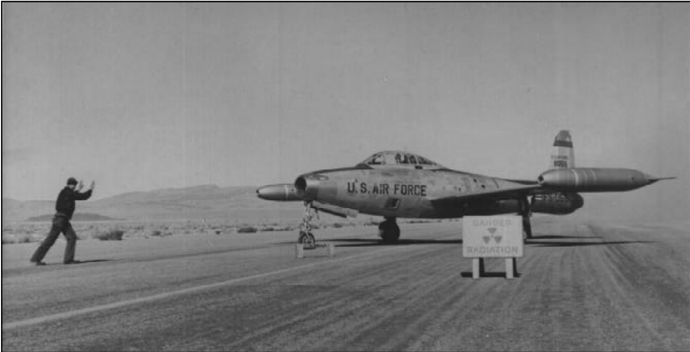
Air Force F-84 being directed to a holding area to await decontamination. The aircraft had been on a cloud sampling mission. Upon landing, the aircraft was surveyed for radioactivity and found to exceed acceptable levels.
