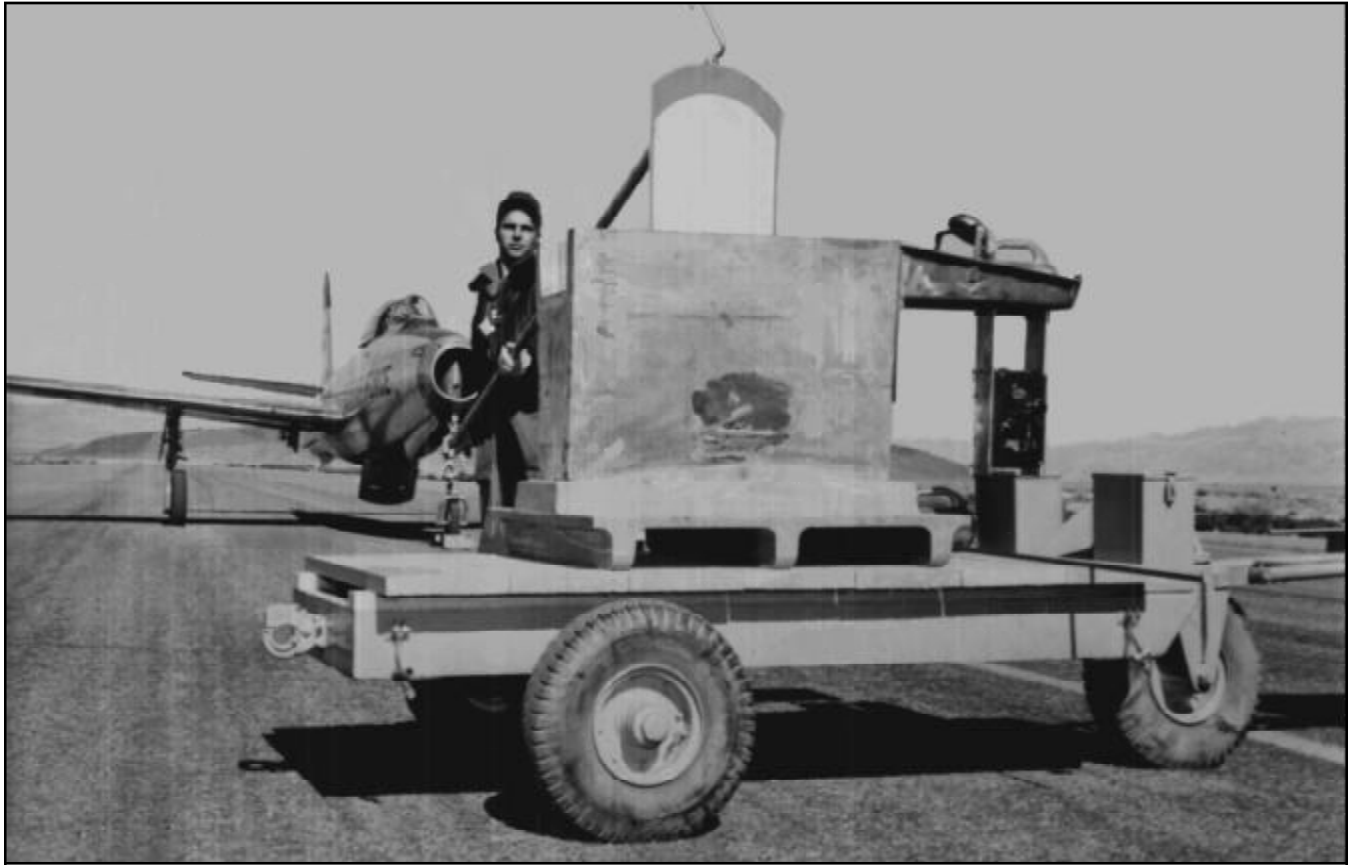
Cloud sampling filter being placed on a cart after being removed from a F-84 sampling aircraft
