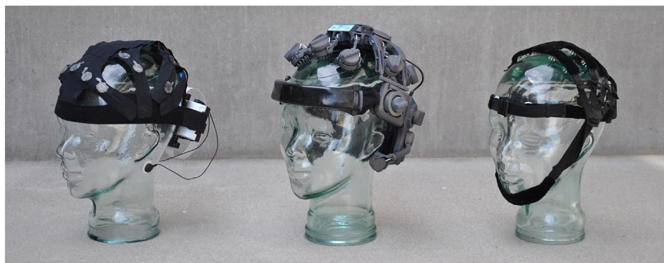
Fig. 5. Three dry-electrode EEG caps designed and tested under the CT2WS program. (Left) B-Alert X24 Wireless EEG Headset System designed by Advanced Brain Monitoring, Inc. (ABM), with 24 standard wet sensors replaced with semi-dry, hydrogel-based sensors. (Middle) Dry-electrode EEG system developed by Quantum Applied Science and Research, Inc. (QUASAR), containing 20 hybrid resistive-capacitive dry-electrode sensors. (Right) EEG system developed by researchers at the University of California at San Diego (UCSD), containing 32 dry-electrode sensors in a soft, adjustable headset.
